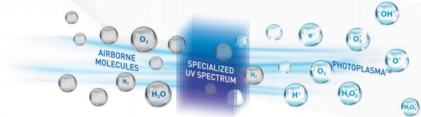
PhotoPlasma<sup>™</sup> is generated by airborne molecules such as oxygen and water vapour under the exposure of the specialized UV spectrum. It includes reactive oxygen species, free radicals, electrons, etc., which actively capture various air contaminants, and rapidly destroy their structures through a chain of reactions. In this way the contaminants are decomposed and converted into harmless end-products like carbon dioxide and water.
